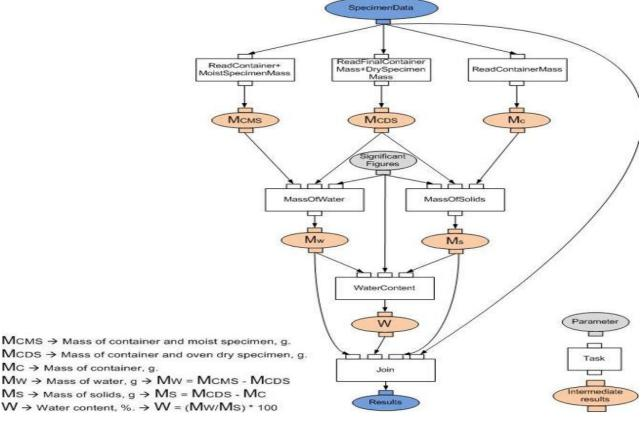
Fig. 4. ASTMD2216-5122 Protocol as Workflow
